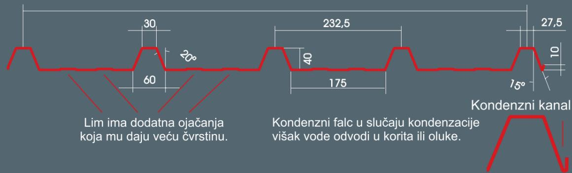
ISPITIVANJE UGLEDA NA SAVIJANJE S ODREĐIVANJEM DOPUŠTENIH OPTEREĆENJA ZA  $\sigma_{dop}=140 \text{ N/mm}^2$  i  $w_{dop}=l/200 \text{ mm}$
